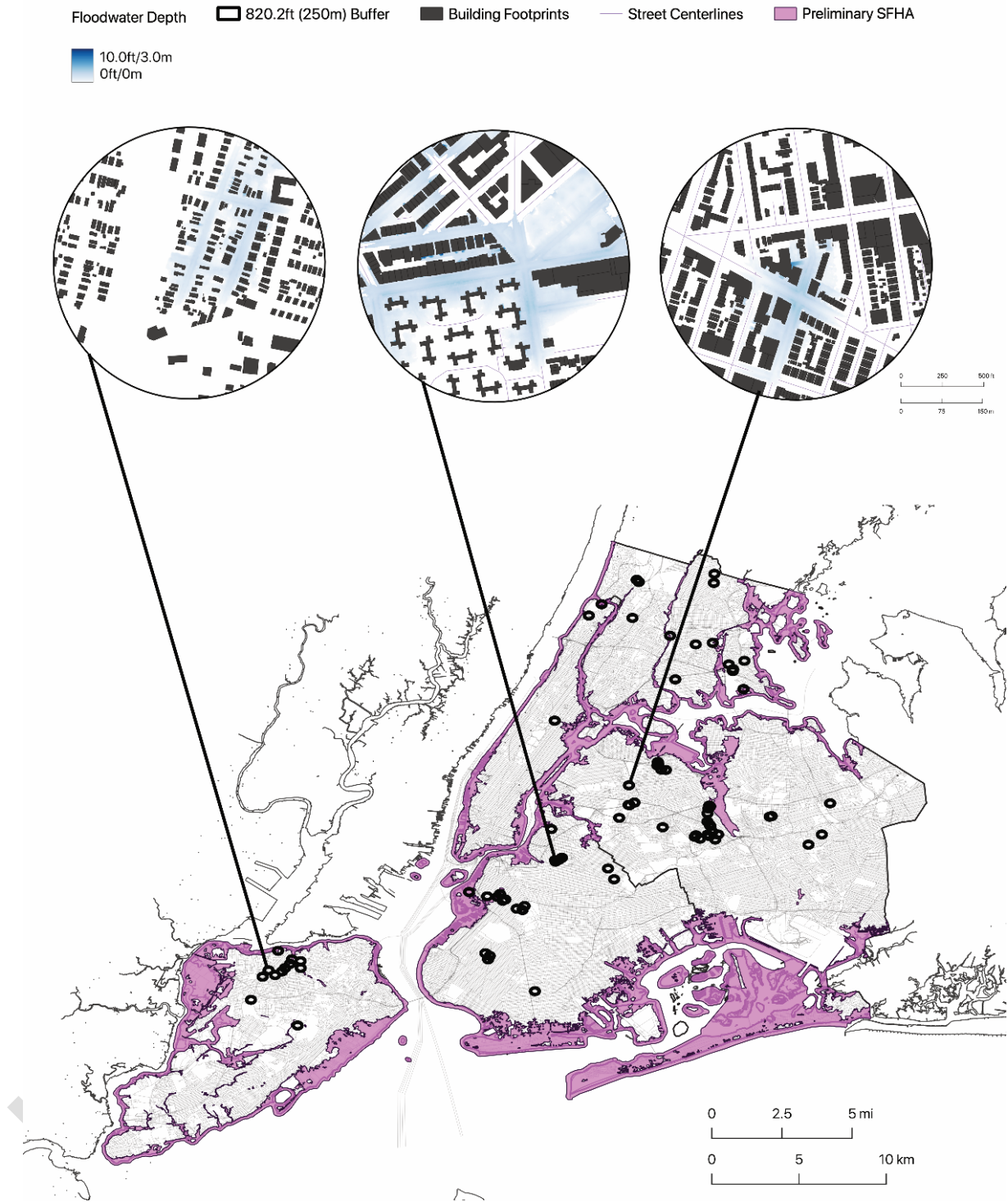
Figure 7: 83 high water marks (HWM) such as seed lines, mud, and debris were surveyed by the US Geological Survey in the weeks following the Ida-Remnants Cloudburst. (Finkelstein et al., 2023) Using these observations, land surface inundation was estimated within an 820.2 ft (250m) buffer of each observed HWMs. During the Ida cloudburst, deep inundation from pluvial flooding occurred in areas that were far from the water bodies used as the basis of FEMA SFHA modeling. Flooding from this event was not limited to areas where HWMs were obtained, and also occurred in areas of the city that were not surveyed or where HWMs could not be identified. Several inundated areas are highlighted here and all HWM data from this survey can be viewed at: https://stn.wim.usgs.gov/fev/#2021lda . Map by BR Rosenzweig.
