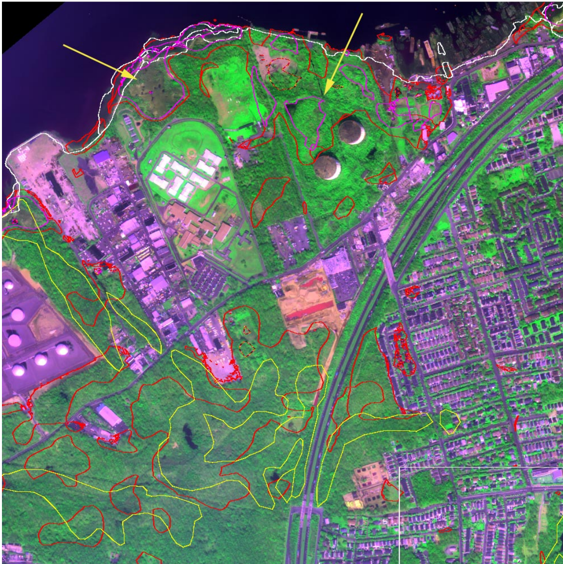
Figure 10a Wetland extents from NYSDEC and DRM bounding extents superimposed on visible-infrared WorldView-2 image from April 23, 2010. NYSDEC tidal (white) and freshwater (yellow) boundaries fail to capture the large potential wetland upper left or the late greening patches upper center (yellow arrows). The DRM extents (magenta=Min, red=Max) show very different coverage from the DEC freshwater extents for the forested area in the lower left
