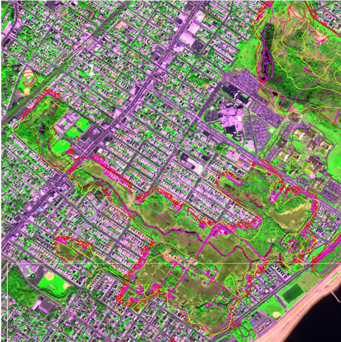
Figure 12a Wetland extents from NYSDEC and DRM bounding extents superimposed on visible-infrared WorldView-2 image from April 23, 2010. NYSDEC tidal (white) boundaries and DRM extents (magenta=Min, red=Max) agree reasonably well but both lap onto the edges of developed areas. Presumably these areas were developed more recently.
