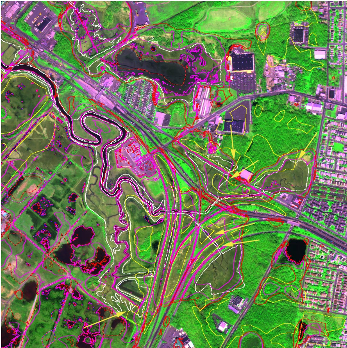
Figure 8a Wetland extents from NYSDEC and DRM bounding extents superimposed on visible-infrared WorldView-2 image from April 23, 2010. NYSDEC tidal (white) and freshwater (yellow) boundaries distinguish the main creek channel and adjacent flats but the freshwater extents do not capture the ponds (left center). The DEC freshwater and tidal extents overlap in several locations (see yellow arrows) The DRM extents (magenta=Min, red=Max) capture both freshwater and tidal wetlands consistently but does not distinguish between them.
