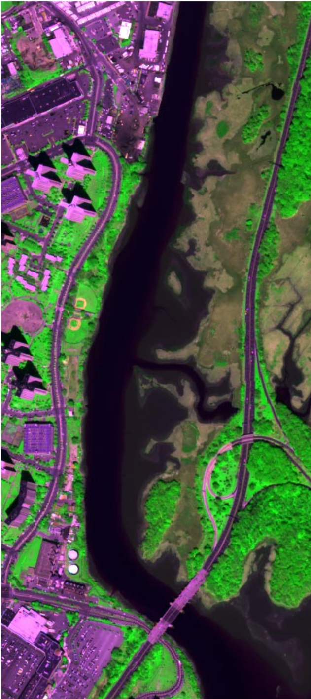
Figure 1 Pelham Bay Park and Co-Op City as seen by WorldView-2 and Landsat 5. With 2 meter spatial resolution WorldView-2 can resolve individual buildings, cars, roads and trees. With 30 meter resolution Landsat 5 does not resolve these small features but it does detect the light reflected from them as it contributes to the spatially averaged color of the pixel containing the features. In these images, the green channel corresponds to Near Infrared brightness rather than visible green. This causes vegetation to stand out in greater contrast to other materials. These images were acquired one day apart in late April 2010 before wetland grasses had emerged so wetlands appear brown.
