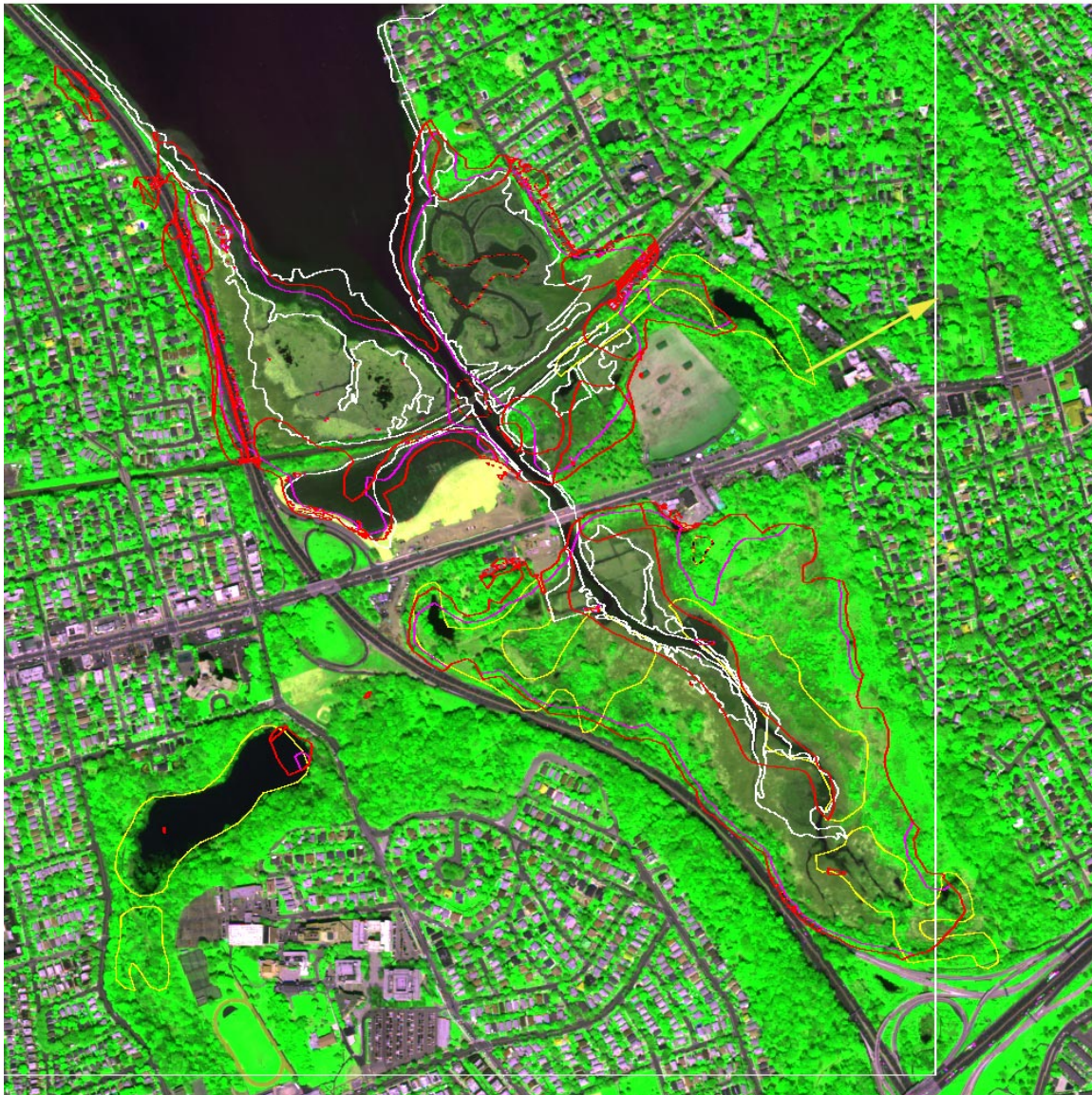
Figure 15a Wetland extents from NYSDEC and DRM bounding extents superimposed on visible-infrared WorldView-2 image from April 23, 2010. NYSDEC tidal (white) appear to underestimate the extent in many areas while freshwater (yellow) etents also do not extend into the darker soils. In oontrast, the DRM exents (magenta=Min, red=Max).extends well into the partially forested area
