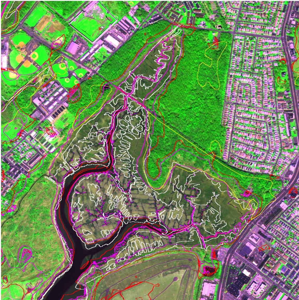
Figure 7a Wetland extents from NYSDEC and DRM bounding extents superimposed on visible-infrared WorldView-2 image from April 23, 2010. NYSDEC tidal (white) and freshwater (yellow) boundaries distinguish different classes of wetland with reasonable accuracy but do not capture the mud flats on the main channel or the late greening area in the lower left. The DRM extents (magenta=Min, red=Max) capture the mud flats exposed at low tide and the smaller late-greening areas at center-upper left. The maximal extents (red) do not capture some isolated freshwater patches in the forest surrounding the creek and misidentify areas on the landfill center bottom.
