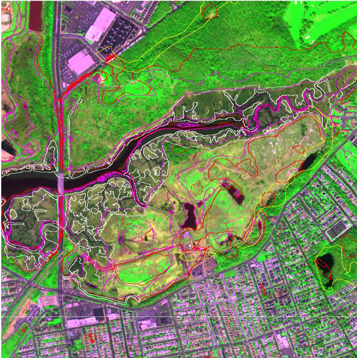
Figure 6a Wetland extents from NYSDEC and DRM bounding extents superimposed on visible-infrared WorldView-2 image from April 23, 2010. NYSDEC tidal (white) and freshwater (yellow) boundaries distinguish different classes of wetland with reasonable accuracy but do not capture some pools further from the creek and extend into developed area in upper left-center. The DRM extents (magenta=Min, red=Max) capture the mud flats exposed at low tide as well as more densely vegetated areas further from the creek.
