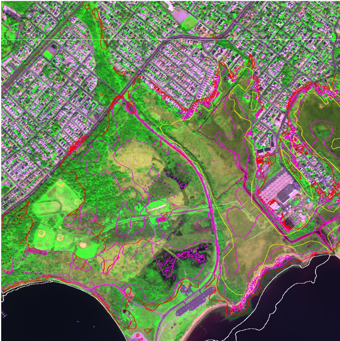
Figure 11a Wetland extents from NYSDEC and DRM bounding extents superimposed on visible-infrared WorldView-2 image from April 23, 2010. NYSDEC tidal (white) boundaries are displaced more than 100 meters offshore (lower right) - even on this low tide image. Freshwater (yellow) boundaries miss the large area of wet soil and standing water surrounding the ballfields and the panhandle on the north side of the park. The DRM extents (magenta=Min, red=Max) capture the extent of the wet soil accurately.
